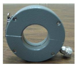
The F-61 is for laboratory and field testing. It is ideally suited for measuring small currents from 10MHz - 1 GHz. This probe has a small outer diameter, approx. 71mm with an internal diameter of 32mm. Its transfer impedance is  $16\Omega$  from 70 MHz to 1 GHz. It can an operate up to 200 amperes of DC – 400Hz, 20 amperes of CW and 50 amperes of peak pulse.
